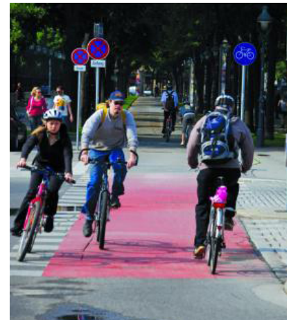
Painted crossing on a bike path in Vienna, Austria.
