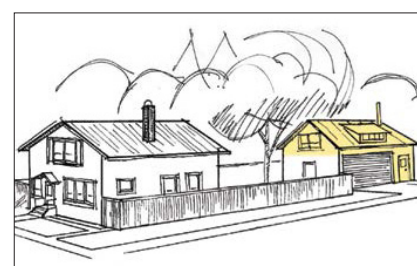
Figure 10: Garage Suite (also called Coach House): Dwelling build above or attached to a detached garage. The suite has an entrance separated from the main garage entrance.
