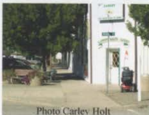
Figure #1: Curb ramp with flares allow access for mobilized scooter
