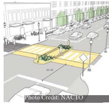
Figure 6: Midblock raised crosswalk
